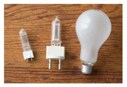
The oldest light source around is the tungsten, incandescent light bulb. They have a wire filament inside that produces the light. They are rated at 2700 – 3400 Kelvin (warm, yellow light). This is a very clean light – not green at all. The lower wattage bulbs have a fitting that is a standard light bulb fitting called an Edison base (E26) pictured left.
